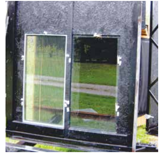
Glass panes are being tested at the Powdermill Tunnel, as seen from the outside. Photo by Christine Sheppard, ABC
